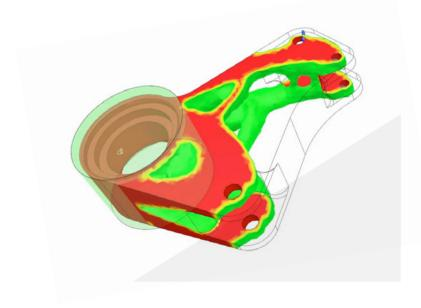
Topology optimization is a familiar technique for most engineers that has gained new life with the possibilities of additive manufacturing.
