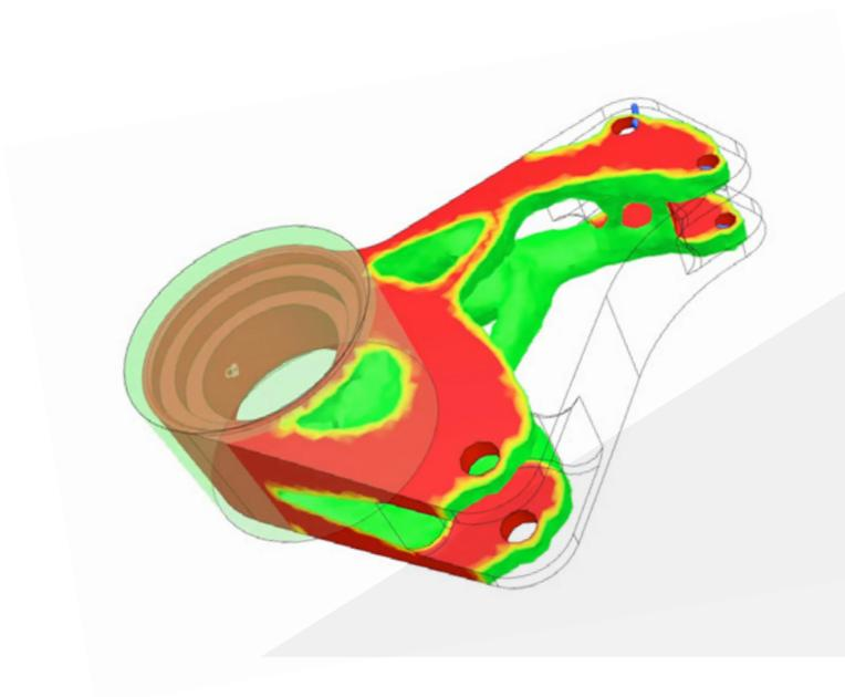
Topology optimization is a familiar technique for most engineers that has gained new life with the possibilities of additive manufacturing.
