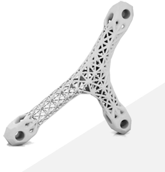
Instead of solid structural beams, the generatively designed seat frame has a bridge with hundreds of smaller lattice cells and several thousand small struts that vary in thickness to bear local loading conditions.
